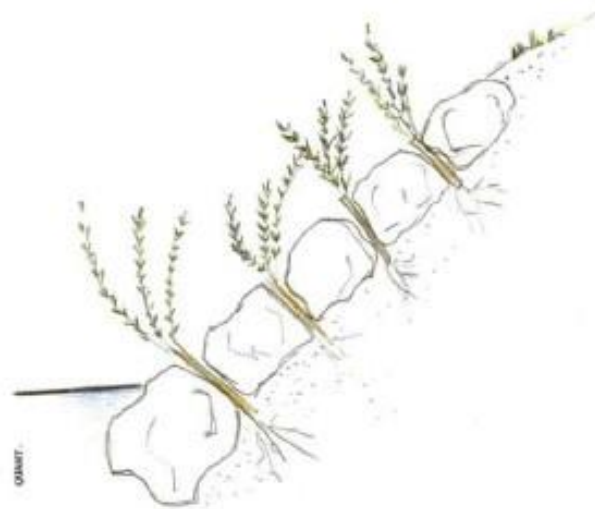
Figure 4.5.2. 2 Riprap with live stakes (Paola Sangalli).
